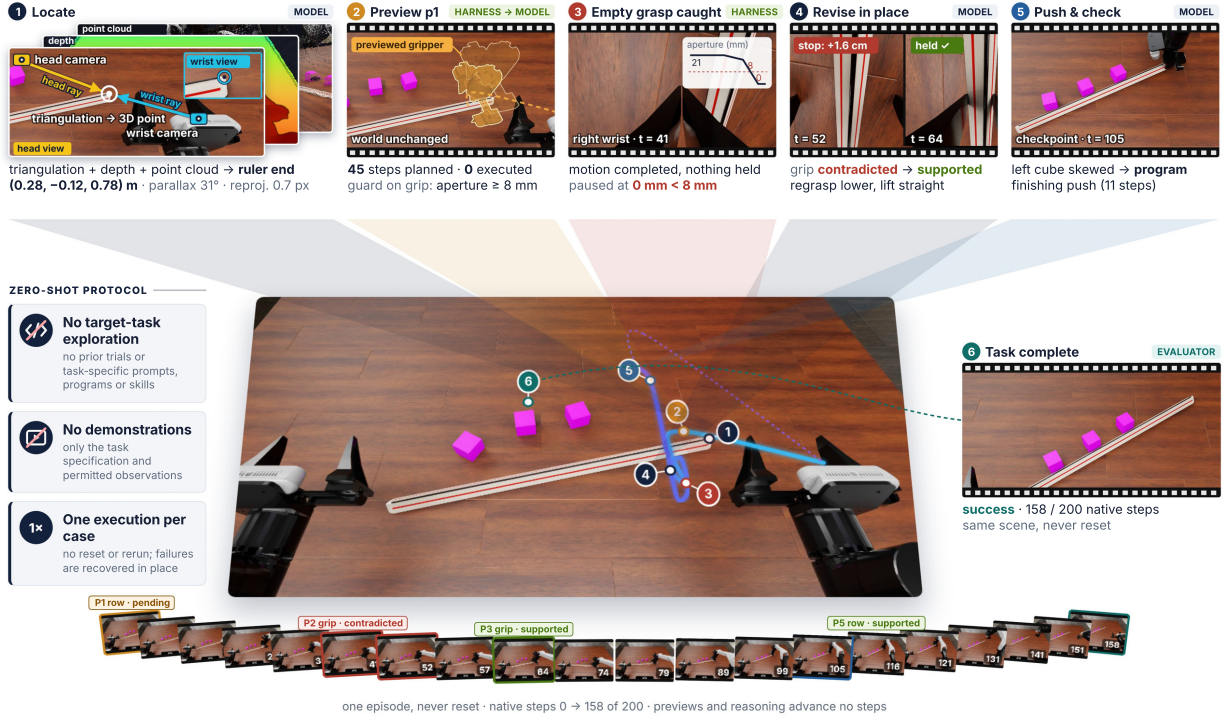
Figure 1 Auriga completes manipulation tasks zero-shot within a single episode. A general-purpose model plans and acts through a shared harness, with no target-task exploration, demonstrations, or resets. The model localizes targets by multi-view triangulation, complemented by depth and point-cloud estimates (1), and reviews candidate motions before they are executed (2). The harness verifies each execution and stops when an action fails (3); the model then revises its plan and recovers from the current state (4–5) until the task succeeds (6).
